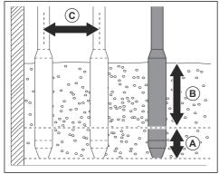
Wait approximately 10–20 seconds until the surface around the vibrator head is shiny and no air bubbles come to the surface.
