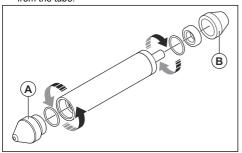
**Note:** The end cap has a right hand thread. The tube connector has a left hand thread.
