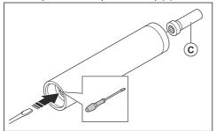
3. Remove the eccentric element (D) and the 2 bearings (E) from the tube.
