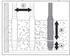
Wait approximately 10–20 seconds until the surface around the vibrator head is shiny and no air bubbles come to the surface.
